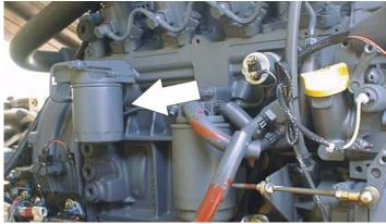
Lube Point(s) - Fill Cap/Spin-on Element Capacity - 11 Quarts Crankcase; 5 Quarts Cooler Lube - EO Interval - Every Year or 1200 hours of operation Comments - Check level daily/Change in accordance with engine manual. 16. Oil Change w/Filter - Caterpillar
