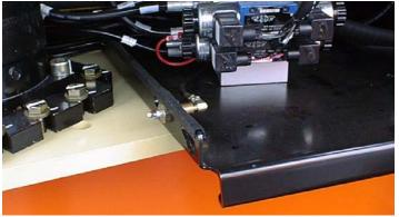
Lube Point(s) - 2 Grease Fittings Capacity - A/R Lube - MPG Interval - Every 3 months or 150 hrs of operation Comments - Remote Access
