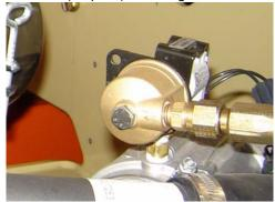
Interval - 3 Months or 150 hours of operation Comments - Replace filter. Refer to Section 6.7, Propane Fuel Filter Replacement
