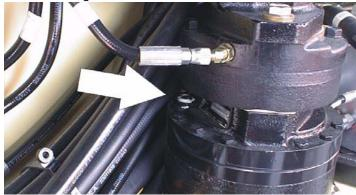
Lube Point(s) - Level/Fill Plug Capacity - 17 oz. (1/2 Full) Lube - EPGL Interval - Check level every 3 months or 150 hrs of operation; change every 2 years or 1200 hours of operation 7. Wheel Drive Hub
